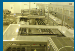
CLEAN PANS MOVE ON TO THE MOULDERS.
